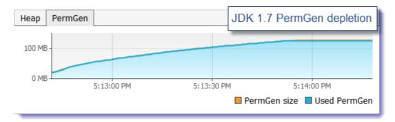
As you can see form JVisualVM, the PermGen depletion was reached after loading about 30K+ classes. We can also see this depletion from the program and GC output.
